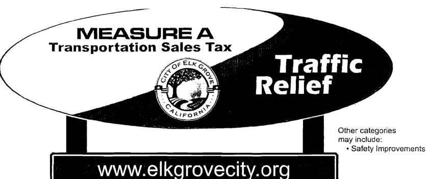
Signs are to be oval shaped and approximately 10'x3.5' on highways and 5'x1.75' minimum for local projects, mounted on 4"x6" min. wood posts (smaller blue sign optional)
