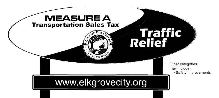
Signs are to be oval shaped and approximately 10'x3.5' on highways and 5'x1.75' minimum for local projects, mounted on 4"x6" min. wood posts (smaller blue sign optional)
